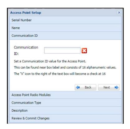
The Communication ID is the 16 digit alpha-numeric number of the Zigbee module inside the access point and can be found on the Access Point near the box label.
